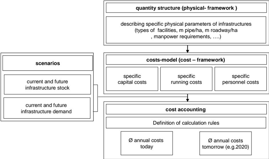
Figure 5: Structure of the infrastructure cost calculation tool
