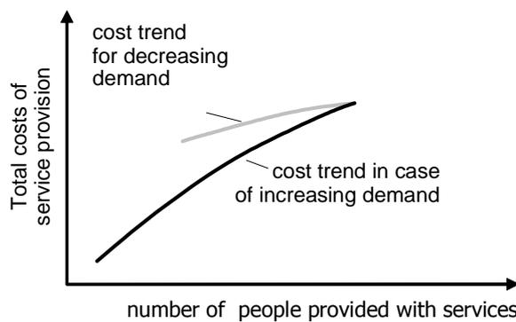
Figure 3: Persistence effect on costs for infrastructure services even while demand is decreasing. Source: Junkernheinrich/Micosatt 2005 (modified)
