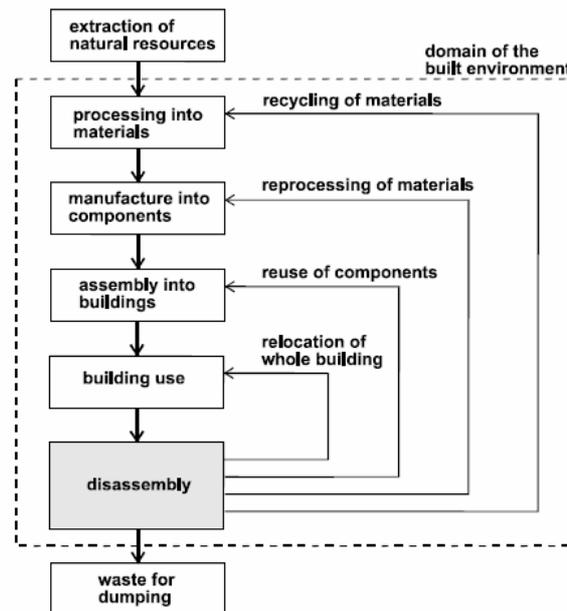
Figure 4 Life-cycle of materials using design for disassembly (Crowther 2000a)
