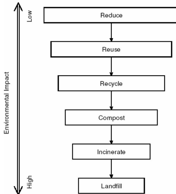
Figure 2: Hierarchy of construction and demolition waste disposal (Peng, Scorpio and Kibert 1997)
