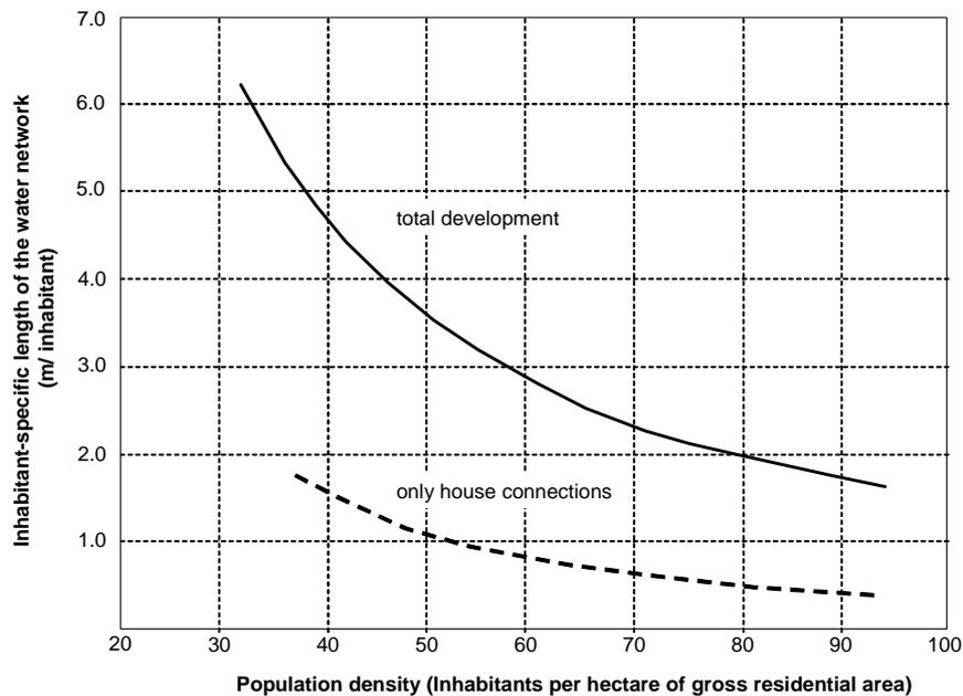
Figure 1 Network length of water provision in relation to urban density, illustrated by the example of Erfurt, Germany. Source: Schmidt 2000 (modified)
