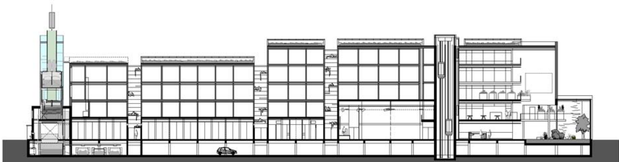
Figure 3: Longitudinal section over the EVA Centre with integrated Sustainable Implant (left).
